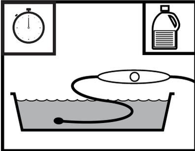
7. After waiting for the disinfectant's specified soak time, rinse the endoscopic shaft and scan head with room-temperature running water for a minimum of three minutes. Do not rinse the controller or cable. Some disinfectant manufacturers may recommend additional rinsing. See the manufacturer's guidelines for more information.
