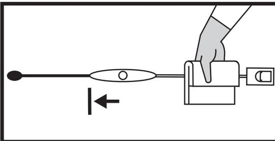
3. Use a second clean cloth moistened with water to wipe the endoscopic shaft and scan head. Be sure to remove all visible biological material.
