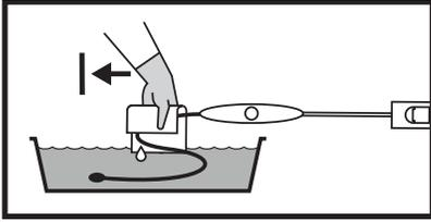
7. After waiting for the cleaner's specified soak time, rinse the endoscopic shaft and scan head with room-temperature running water for a minimum of three minutes to remove residual cleaning solution.
