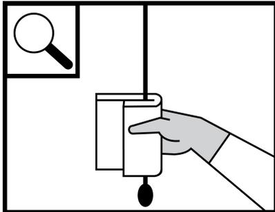
10. Inspect the transducer and cable a second time for any sign of damage that might have been overlooked during your initial examination or that was previously obscured by biological debris. If damage is evident, discontinue use of the transducer and contact FUJIFILM Sonosite or your local representative.
