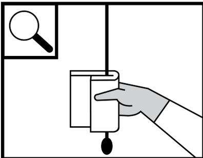
9. Inspect the transducer for damage, such as cracks or splitting where fluid can enter. If damage is evident, discontinue use of the transducer and contact FUJIFILM Sonosite or your local representative.
