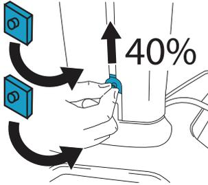
4. Slide another single nut pad up into the column and then secure the printer shelf with the 4mm hex key and two M5 hex screws.
