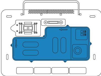
2. Place one of the batteries in the compartment as shown, then plug its cable into the connector. Make sure the cable is placed fully within the compartment.
