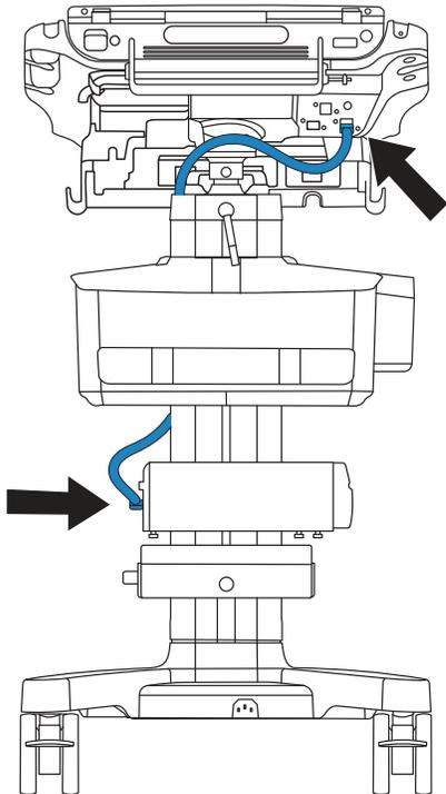
5. Connect the column power cable to the stand head by pushing it into place and screwing it into the connector. Tug gently to make sure it is secure.
