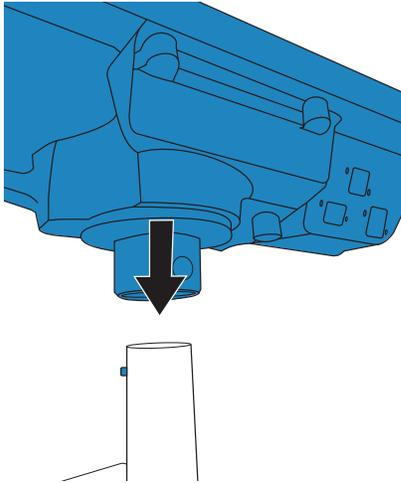
2. Use the security screw and 5/32 security hex key with the central hole to tighten the stand head to the post.
