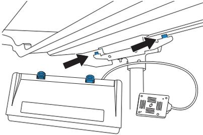
2. Insert screws, with insulating washers, through the screw holes in the stand head. Lift the TTC with your hand as you tighten the screws with the 2.5 mm hex wrench provided in the TTC installation kit.
