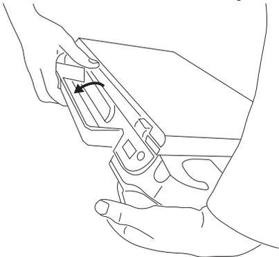
5. Connect the TTC connector to the system by placing the docking connector in the recess and turning the latch. Then fold the latch down.
