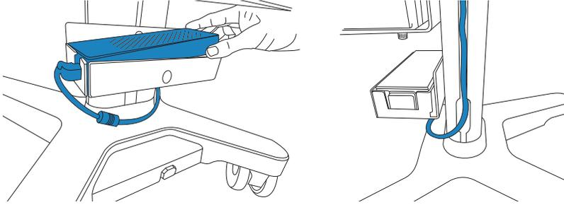
10. Plug the shorter cable coming up through the stand into the power supply.
