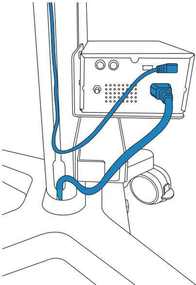
9. Place the power supply into the tray and then run the connected cable under the tray and up through the channel in the side of the stand.
