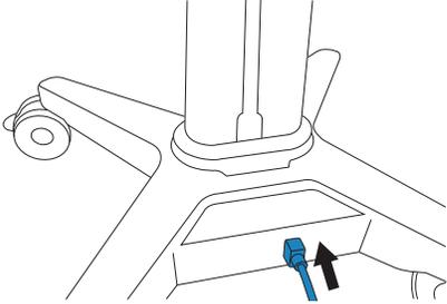
2. Run the AC power cord through the cord clip on the back of the storage tray. Alternatively, install the lower AC cord hook in the following steps. Both serve the same purpose. Wrap the cord if you need to wheel the system to an outlet.
