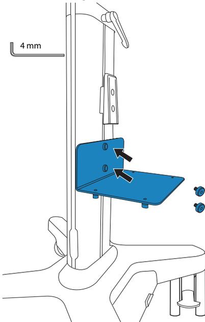
5. Set the printer on the shelf and then use the four thumb screws to secure it. The left thumbscrews use the holes at the rear edge of the printer. The right screws go through the rubber foot pads.
