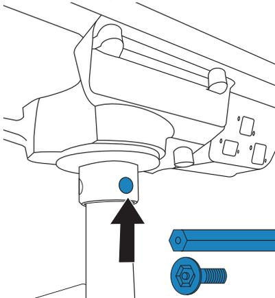
3. Use the same 5/32 hex key to tighten the two preinstalled screws in the collar.
