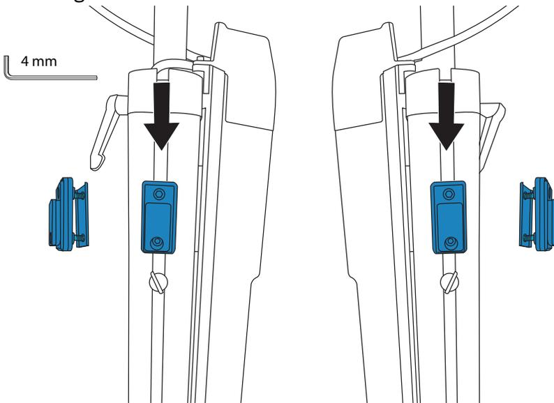
7. Slide the mount down until it is just below the top of the rear storage bin and then tighten both hex screws. Do this on both sides.
