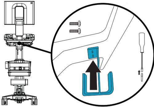
2. Insert the FUJIFILM Sonosite ECG Module into the rear, or stand side, of the mounting bracket. The front of the bracket is for cord storage.
