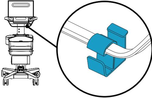
2. Insert the FUJIFILM Sonosite ECG Module into the rear, or stand side, of the mounting bracket. The front of the bracket is for cord storage.
